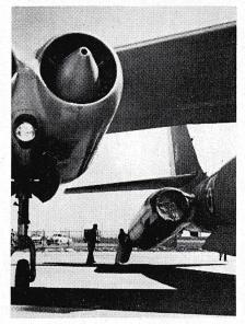
its proximity to the stabilizer. The nacelle was extended about seven feet in front of the engine intake so that baffles could be fitted. These straighten out the airflow reaching the intake. They may also be moved to examine the effect of changes in the direction of airflow into the engine.
