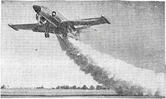
Up She Zooms—Canada's long-range all-weather interceptor jet fighter, the CF-100 Canuck, is seen during a jet-assisted takeoff at RCAF station, Uplands, where it is being tested by the RCAF. Jato cuts normal take off run in half giving CF-100's two Orenda engines an added thrust of 1,000 pounds each.
