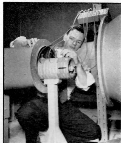
Above, tests being made on airflow characteristics of model turbojet intake, in Orenda Engine's Sir Thomas Sopwith Gas Turbine Exper. Lab.
