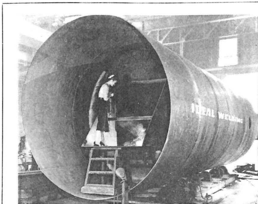
DOES YOUR WIFE TALK TOO MUCH? Shown is one of two jet engine silencers recently completed for Orenda's Nobel facility. Described as being biggest mufflers ever made in Canada, they have 45 ft. length and 11 ft. diam. Made entirely of metal parts, units cut noise to level not exceeding average in surrounding area (70-80 decibels @ 1,500 ft.). They were designed by Industrial Acoustics Co. of New York and fabricated under contract by Ideal Welding Co. Ltd., Scarborough,
