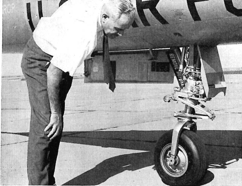
JOHN GELLNER studies the two-position nose-gear of the F-5N.
