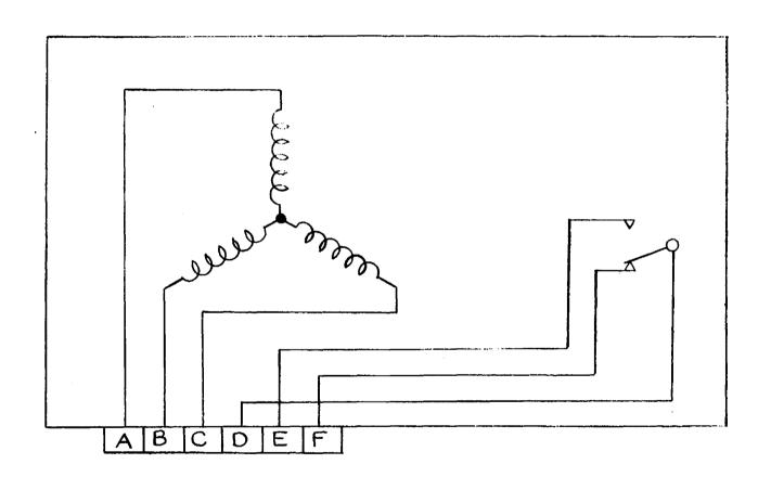
WIRING DIAGRAM-POWER FAILURE DETECTOR.
