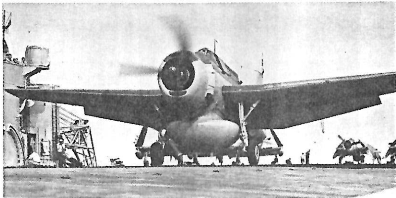
RCN'S NEW GUPPY: Latest version of the versatile Avenger to go into service with the Naval Aviation branch of the RCN is the Avenger 3W2 "Guppy", a flying radar station which the Navy says carries detection gear more powerful than most current shore installations. Though the Guppy does not represent a new concept in airborne early warning, its more powerful radar has enabled new techniques to be devised and has added considerably to the importance of the aircraft's tactical and strategic functions. Fairey of Canada is responsible for the modification program.
