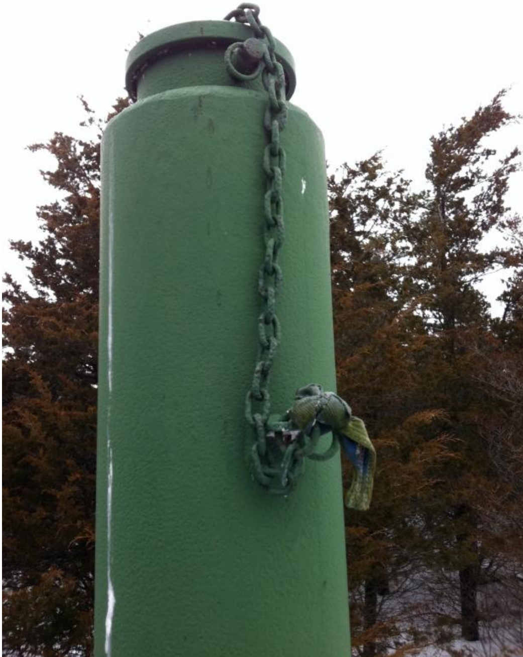
With the paint hardly worn, the 60 year old Orenda jet engine tether test pole looks almost brand new despite sitting exposed to the elements since the 1950s. Tether chain and the rotator cap still remain.
