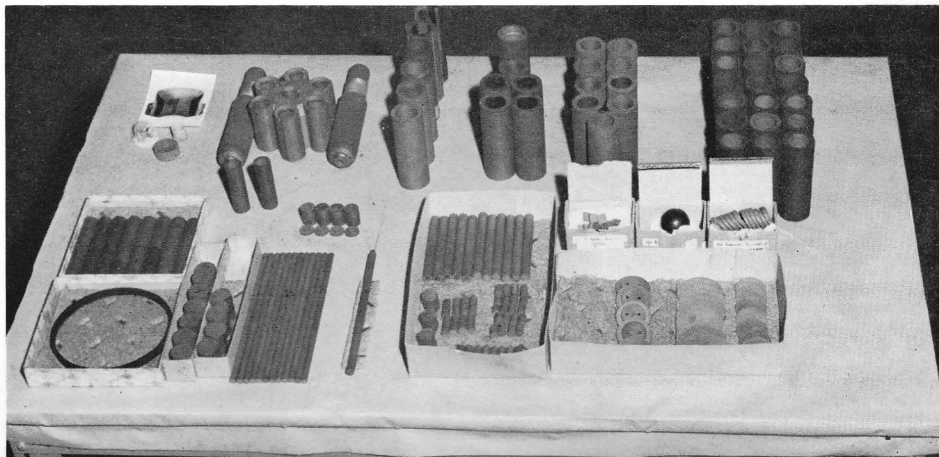
Fig. 2 (above): The apparatus used for impregnating fuel cans. Fig. 3 (below): A selection of graphite components which have been treated to reduce porosity
