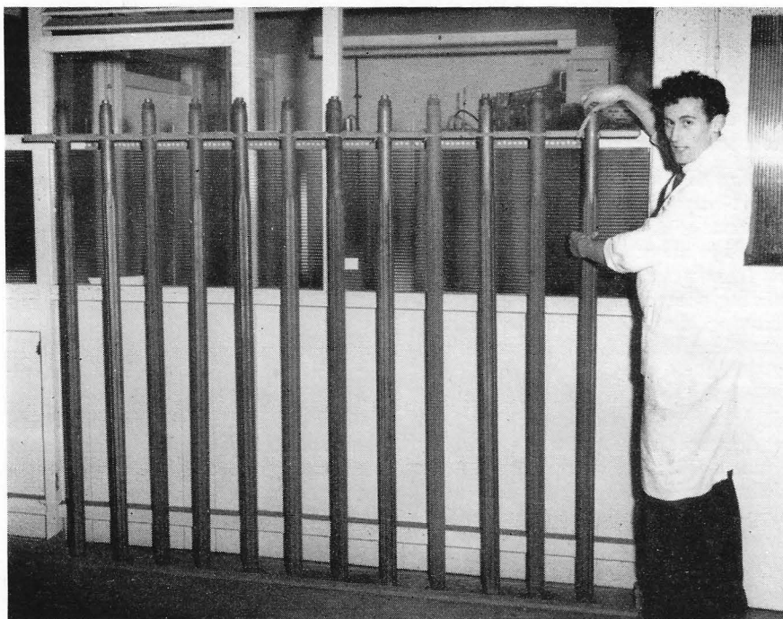
Fig. 1: Graphite fuel cans over six feet (about 2m.) in length can now be treated to reduce their porosity. Essentially the method involves impregnating the graphite with furfuryl alcohol which is then thermally decomposed to leave carbon in the graphite pores
