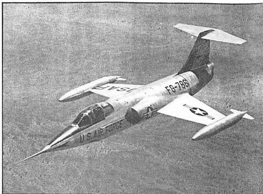
Supersonic aircraft like Lockheed's F-104A (XF-104 shown) are tailored to their powerplants, and vice versa, and are not amenable to engine switches.
