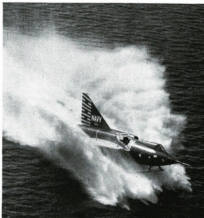
SEA DART, first supersonic fighter to operate off water blazes down a sea lane on a takeoff.
