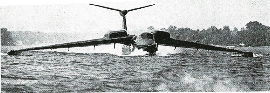
MARTIN SEA-MASTER XP6M-1 with streamlined jet engine nacelles atop wings, fixed plastic wing-tip floats to provide buoyancy in the water.
