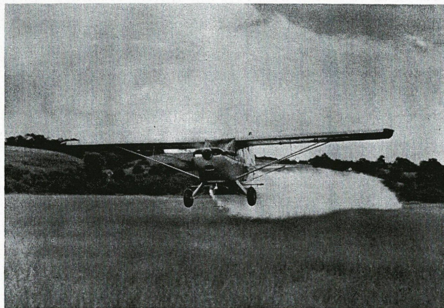
TAYLORCRAFT'S TOPPER is the first fibreglas agricultural airplane. Designed principally for dusting and spraying of chemicals by air, it can also carry five people.
