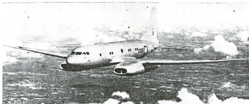
The Avro Tudor 8, the world's first experimental four-jet airliner made its initial flight during September. Powered by four Rolls-Royce Nenes, the Tudor 8 has a service ceiling of 44,000 feet and a maximum cruising speed of 350 mph at 25,000 feet. Its length is 85 feet 3 inches, span 120 feet, height 24 feet, and all up weight 80,000 lbs.
