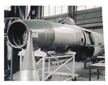
Thames but was abandoned in 1958. This large — length 66ft 6in/20.3m — fighter featured an intake for the engine mounted under the fuselage; beating the General Dynamics F-16 Fighting Falcon to this concept by a full 16 years. The fuselage moved to the College of Aeronautics at Cranfield, Beds, and later went into the care of the RAF Museum.
