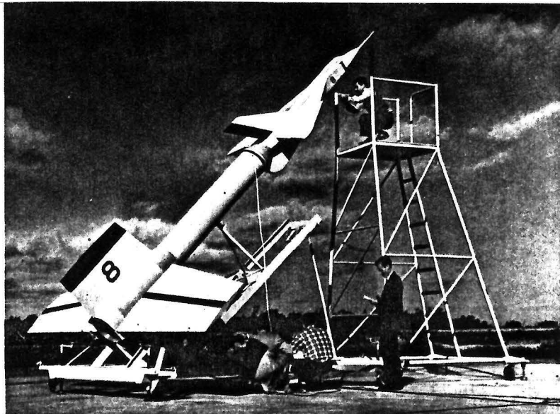
During the long development programme for the CF-105, instrumented free flight models with booster rockets were used to ascertain aerodynamic behaviour at high speeds.
