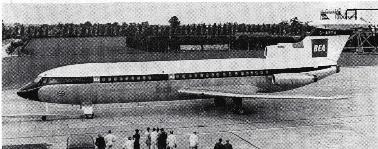
TRIDENT ROLL-OUT. The new de Havilland Trident short-haul jet airliner rolled-out last month, and is scheduled to begin flight trials during the coming winter. Canadian interest in the aircraft centres on it as a possible short-haul vehicle for Trans-Canada Air Lines. The large 12 ft. diameter fuselage will take six-abreast economy seating, accommodating up to 100 people.
