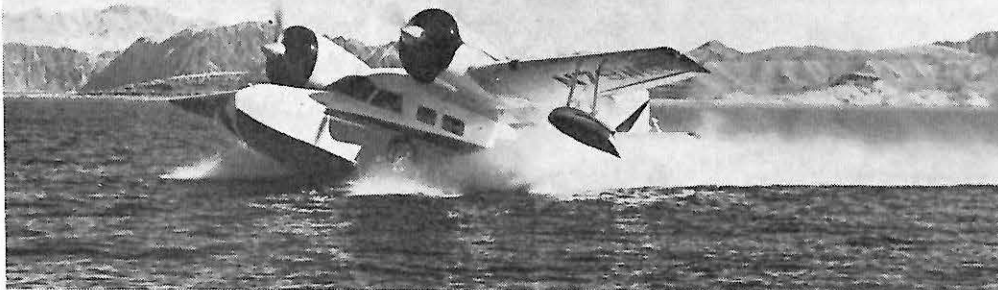
PAGE-CANNET AMPHIBIAN is modernized Grumman Widgeon powered by 300 hp Lycoming R-680's in place of 200 hp Rangers. Cruising speed (66% @ 8000 ft.) is 170 mph; gross weight of modified airplane is 5500 lb.
