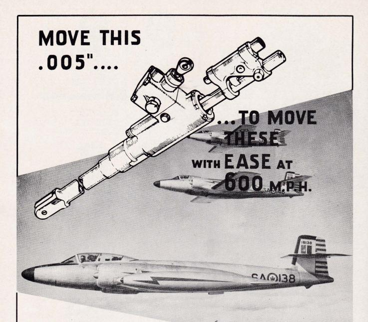
THE problem of control at very high speeds has been largely solved in Canada's CF 100, by the adoption of FAIREY Hydroboosters wherever air loads on the control surfaces are so great as to make manual control arduous.
