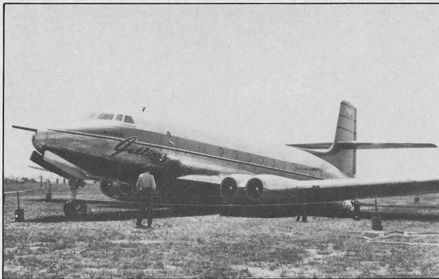
C-102 Jetliner after second flight. Aircraft was belly landed at Malton when the main gear failed to extend. (National Archives)
