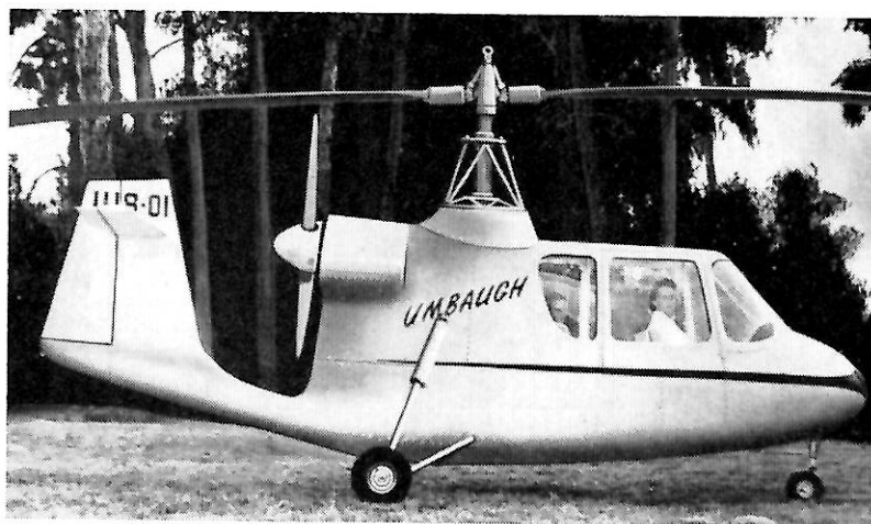
EXECUTIVE GYROCOPTER: Known as the Umbaugh Gyrocopter, this unusually designed two-man helicopter is presently undergoing CAA certification. The Umbaugh is expected to sell for between $8,000 and $10,000 depending upon optional equipment installed. The tiny machine cruises at 100 mph; is powered by a 180 h.p. Lycoming or Continental engine. Avro Aircraft is reported to be studying possibility of producing this aircraft in Canada.
