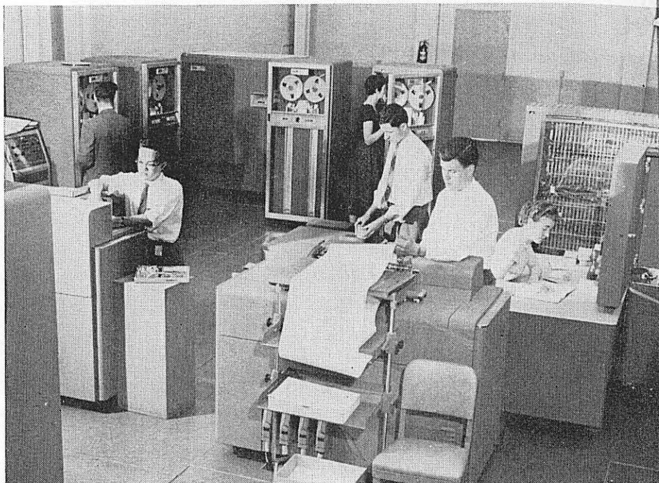
704 LAYOUT. General view of the central area of the 704 computer. Console is at the right, printer output unit is in the foreground, and tape units at the rear.
