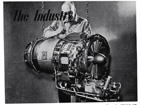
POWERPLANT FOR THE CL-41 trainer is the General Electric CJ610-1B, which will be built in Canada under license by Orenda Engines Ltd., Malton. Canadian General Electric says "close to 250" of the turbojets will be built. The lightweight engine features a very high thrust/weight ratio.
