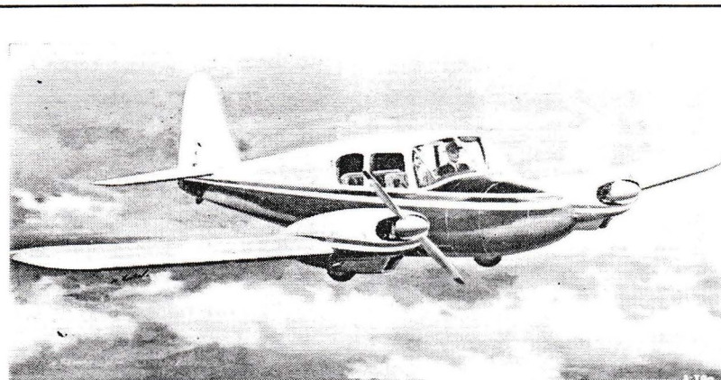
PIPER APACHE: Piper Aircraft Corporation's new twin-engine light transport has been named the "Apache". First production models of the Apache will soon appear and are scheduled to sell for approximately $25,000. Powered by two 150 hp Lycomings, the aircraft will carry four persons at cruising speeds in excess of 150 mph. Full feathering Hartzell propellers are used. Single engine service ceiling in fully-loaded configuration is over 5,000 feet according to Piper.
