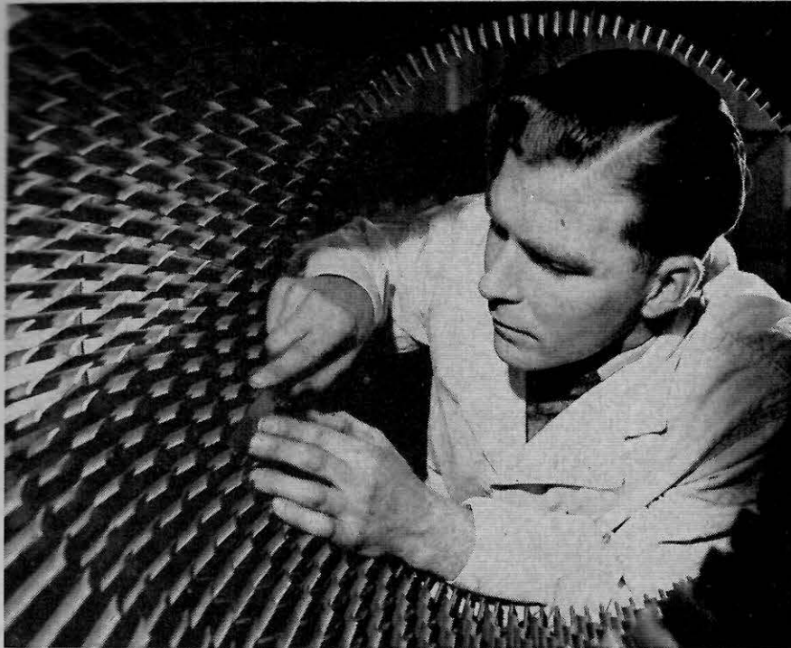
LEFT—Blades have raised the most difficult problems in development of the Orenda jet engine at Avro. John Howlett, engine fitter, is shown scraping and deburring a stator blade.
