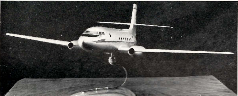
ORIGINALLY Jetliner looked like this, but as specified engines were not available in time the design was changed to the familiar four-jet aircraft we know today.
