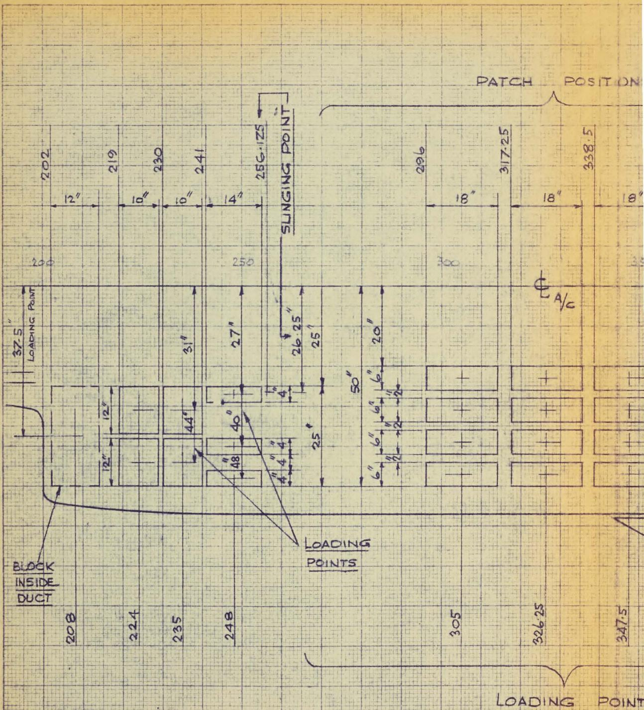
TENSION PATCH POSITIONS ON TOP OF FUSELAGE SINS, 200-
