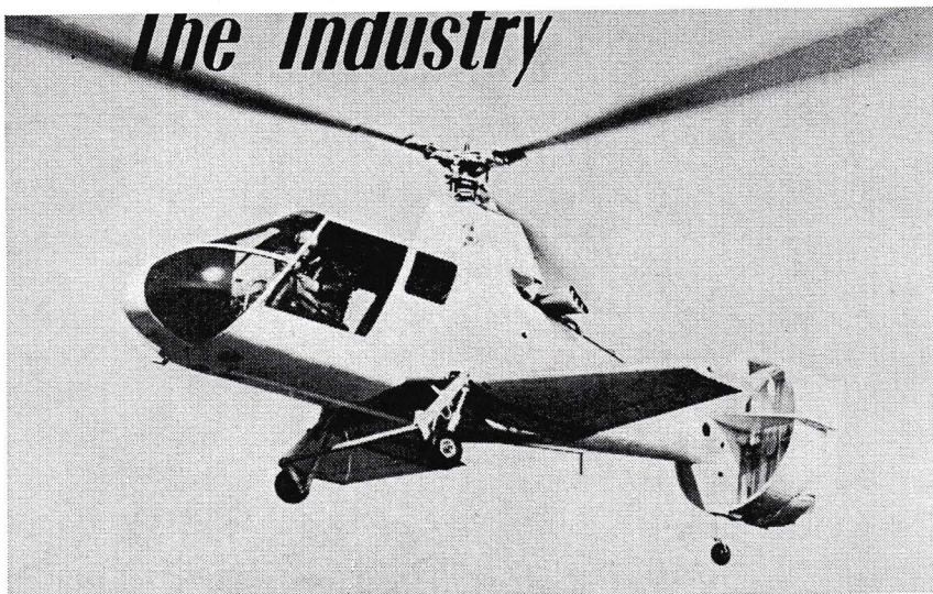
CANADIAN P & W PT6 POWERED Piasecki 16H begins flight tests with wings following completion of tests in pure helicopter configuration. The 16H combines the VTOL and hovering features of the helicopter with the longer range, higher speeds, lower operating costs of the fixed wing airplane.
