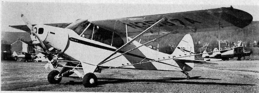
NEW 1954 PIPER AGRICULTURAL PLANE can be used for dust or spray or when equipped with convertible combination unit can be quickly changed for either operation. Powered with a 135-horsepower Lycoming engine, it is equipped with a large tank with capacity for 110 gallons of spray or 18 cubic feet of dust. Safety features include shoulder harness and wire cutters on landing gear. Shown above in sprayer configuration, new 1954 version has larger capacity wind-driven pump relocated forward in prop blast. Booms swing back in case a ground object is struck. 24 nozzles are supplied as standard with booms drilled and tapped for 22 additional nozzles to boost coverage to 15 gallons per acre when desired. PA-18-A is only agricultural airplane in volume production in the world.
