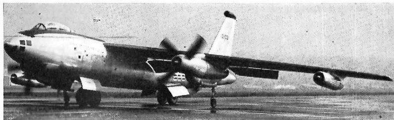
B-47 TURBOPROP TEST BED: This turboprop test vehicle is the Boeing XB-47D, a standard B-47B modified to flight test the Curtiss-Wright T-49 turboprop. Two T-49's are mounted in place of the four GE J-47 turbojet engines normally located at the inboard pod positions. The T-49 is a turboprop development of the J-67 (Wright version of the Bristol Olympus) and is rated at 12,000 eshp. During the test program, the XB-47D retains the two outboard J-47 turbojets of 6,000 lbs. th. each.
