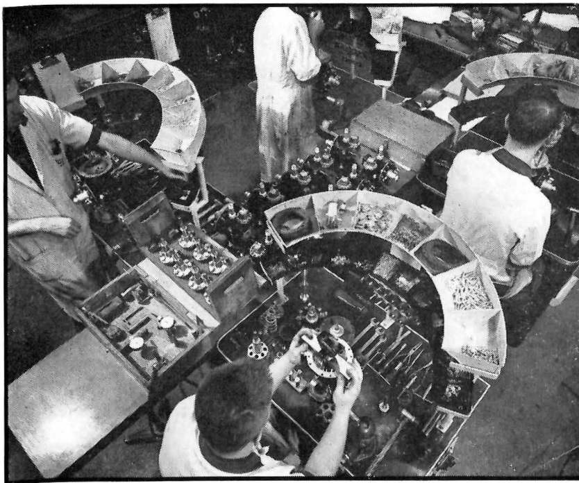
FUEL PUMPS for Orenda engines are shown above being assembled at the Lucas-Rotax plant at Scarborough, Ont. Note fatigue-reducing arc-like arrangement of parts trays. Below is the Lucas-Rotax maintenance plant at Montreal.
