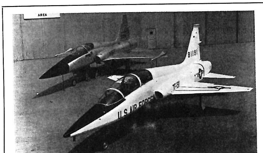
SUPERSONIC TRAINER: First Northrop T-38 supersonic jet trainer is shown on roll-out in mid-August. In background is mockup of new N-156F counterair fighter which Northrop is developing from T-38. The jet trainer is powered by two GE J-85s, weighs 10,960 lbs., combines supersonic climbing speed with landing speed low enough to eliminate need for a drag chute.
