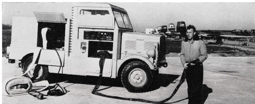
COMBINATION AIRCONDITIONING and A-C power supply unit—part of the Arrow's ground support equipment—is displayed by Alex Cochane of Flight Test. This special unit is designed to maintain the temperature of the electronic equipment at scramble readiness. Once the aircraft's engines are started, the unit's task is taken over by the internal system.
