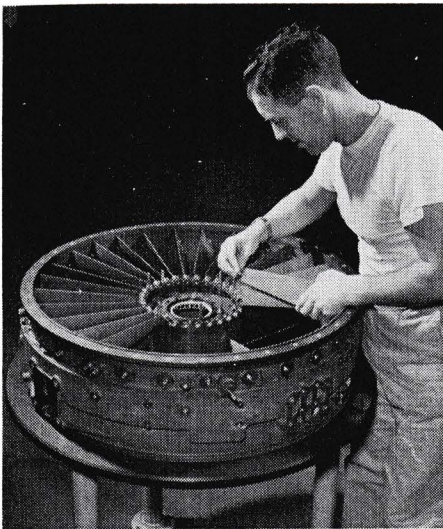
VARIABLE INCIDENCE inlet guide vanes being inserted in front frame of the J-79-7.
