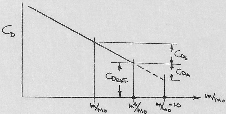
In this report the spillage drag is defined as the drag increment due to spilled intake flows where the intake is running at less than choke mass flow (i.e. the internal drag) and the additive drag is defined as that portion of the external drag due to spilled intake flows when the intake is running full.
