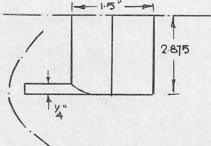
Assume drag of pitot is equivalent to an isolated cylinder and double-wedge aerofoil.
