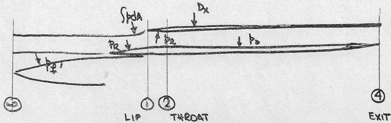
The free-flight model is not utilized to assess the spillage drag, but to give the total external drag, as defined i.e. the shock structure and internal flows should simulate choked thrust flows. The total change of momentum, choked flow, must then be subtracted to give the correct  $C_{D_x}$ .
