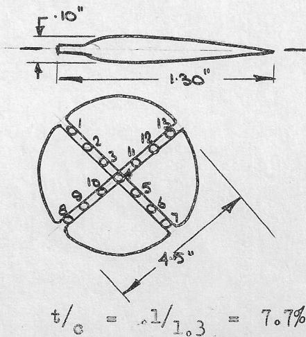
13 pitots imbedded in an aerofoil shape.
