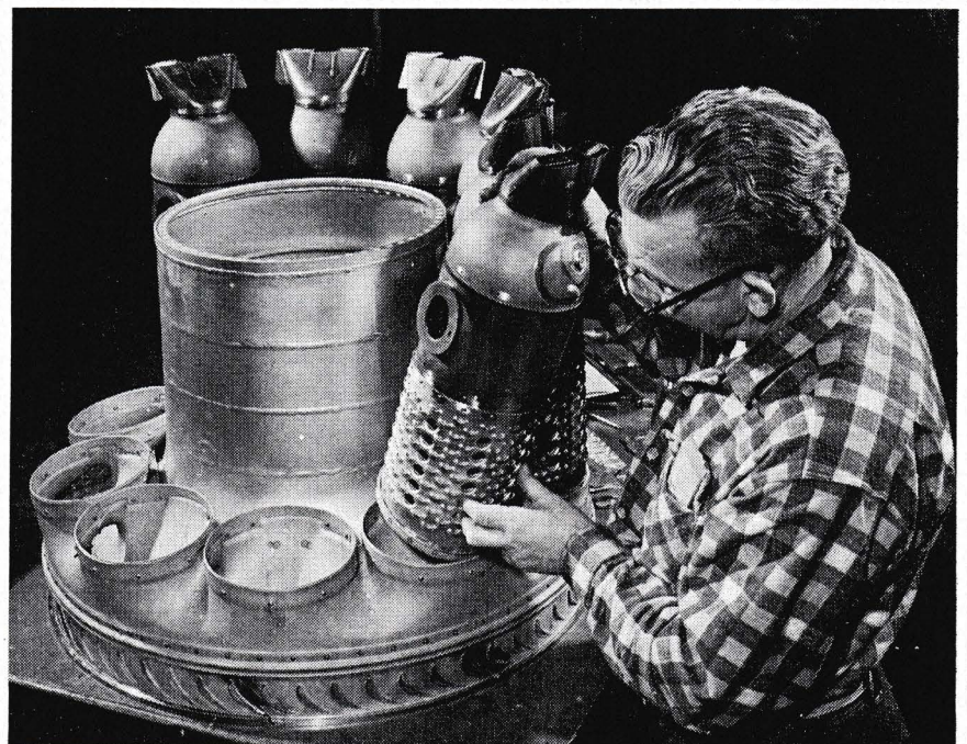
COMBUSTION LINERS being fitted, showing the annular intake and the inner connecting pads for mounting the inner connectors between each of the liners.
