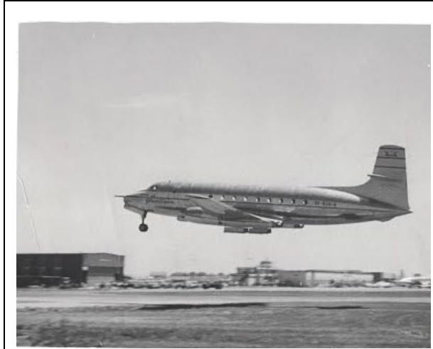
AVRO Jetliner with nose wheel down, mains locked up and no flaps just before belly landing
