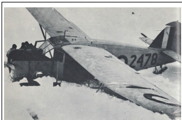
The day after the crash Damage to the left wing is obvious
