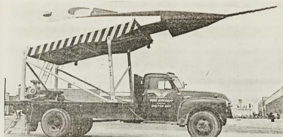
Mock-up of the cockpit was mounted on a truck at actual height and taxiing attitude of the Arrow in order to check pilot visibility under actual daylight and night operating conditions.
