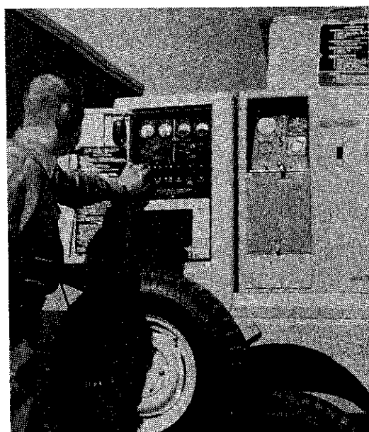
CONTROL PANEL of the starter jeep. Intercom is provided between unit and pilot during starting operation.
