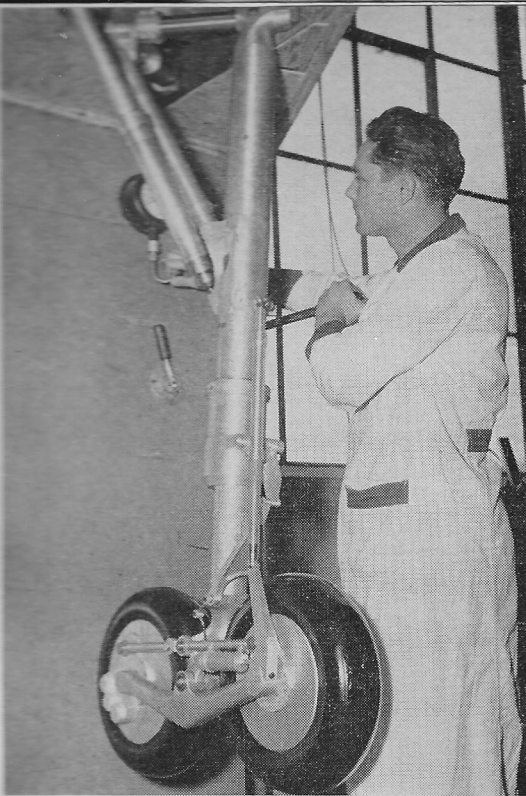
HALF-SCALE working model of the Arrow landing gear provided design assist.
