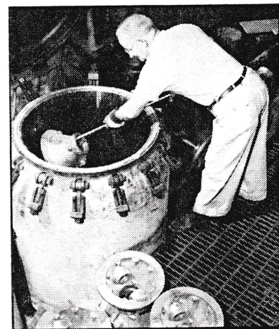
Magnesium gearbox housing for Orenda is placed carefully in Stokes vacuum impregnating chamber by operator at York Gears. Large castings like these are loaded individually; smaller castings in perforated metal baskets.
