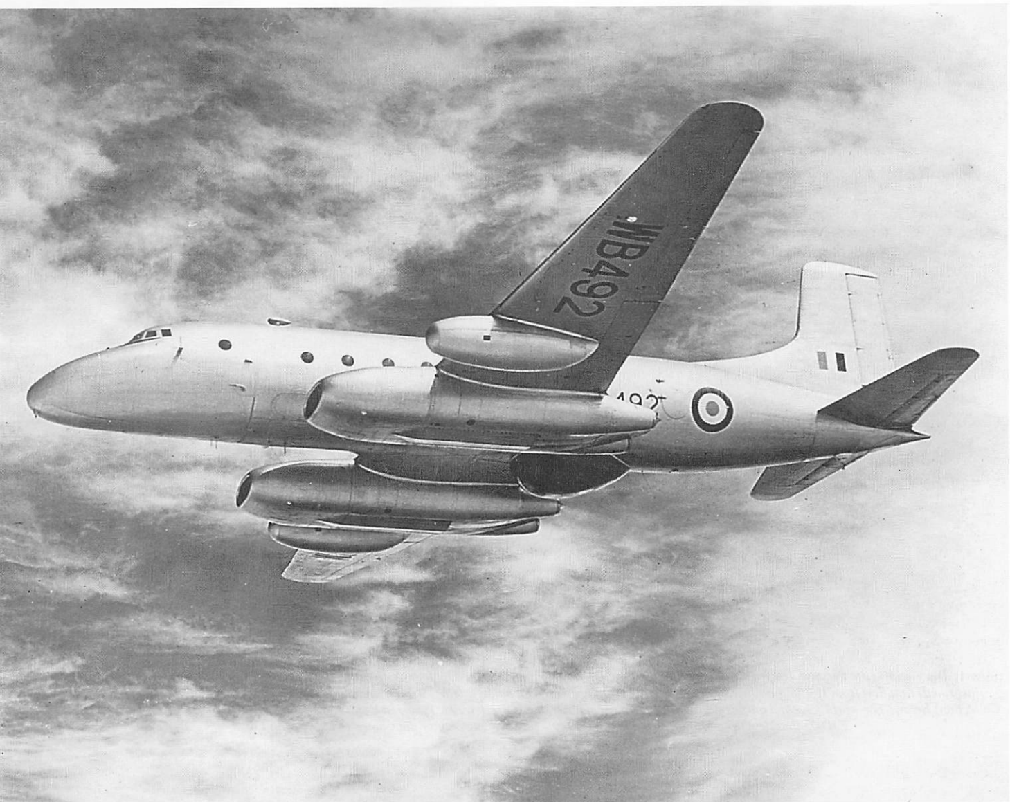
Avro's Type 706 Ashton was a development of the Tudor airliner, via the Tudor 8 powered by four Nenes, for research purposes for the Ministry of Supply. Erroneously compared with the Jetliner (see page 61), the first example flew on September 1, 1950. Illustrated is Mk 3 WB492 used by the Radar Research Establishment. (Don Hannah Collection)
