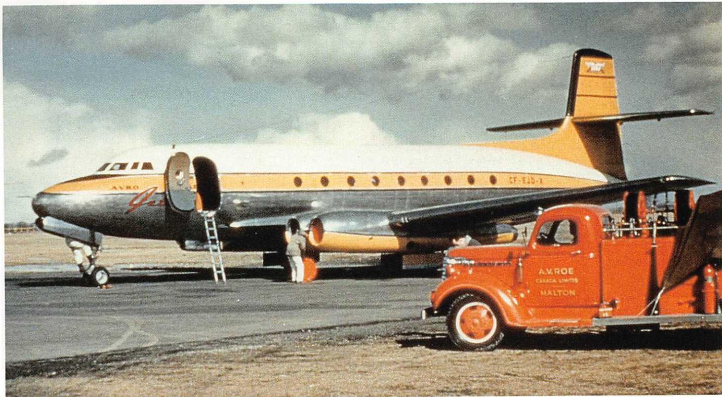
The Jetliner seen at Malton during the early 1950s. Note the de-icing strips on the tail surfaces and the 'white top' fuselage (see front cover). Also, note how accessible the engines were to the mechanics on the ground. (Don Rogers via Jim Floyd)
