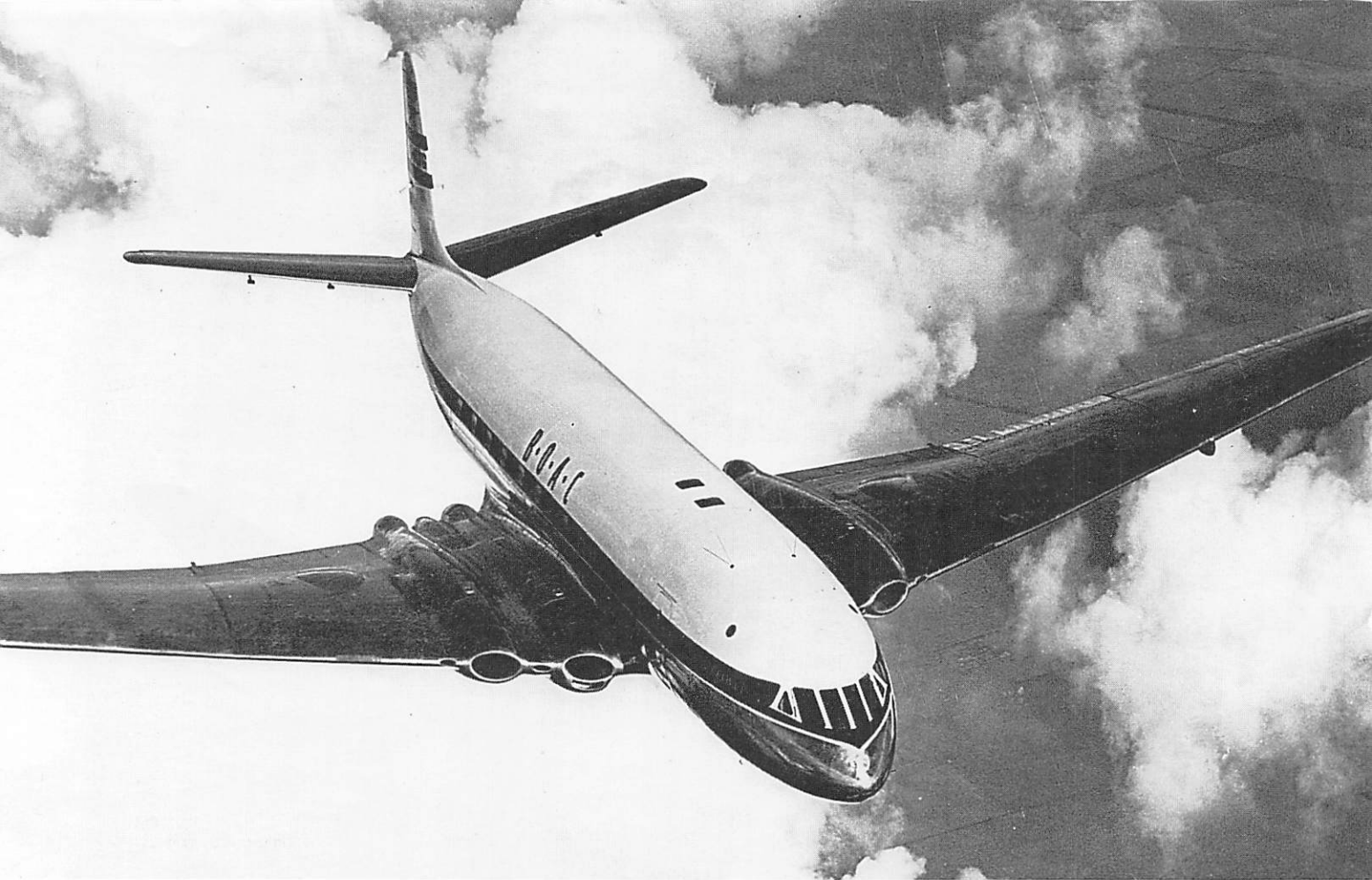
Above: The world's first purpose designed passenger jetliner, the DH.106 Comet. Powered by four de Havilland Ghost 50s, the prototype, G-5-1/G-ALVG (illustrated) first flew from Hatfield on July 27, 1949. Early customers were Canadian Pacific Airlines and the Royal Canadian Air Force. (Don Hannah Collection) Below: The world's second purpose-designed passenger jetliner, the C102 Jetliner. Powered by four Rolls-Royce Derwent 5s, the prototype, CF-EJD-X, first flew from Malton on August 10, 1949 – just two weeks after the Comet. (Avro via Jim Floyd)
