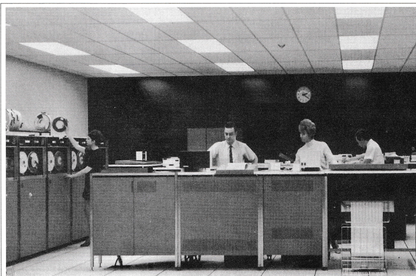
The Data Centre in 1970. At the left, the bank of five tape drives and a printer; in the centre, the card reader, console and second printer. Not seen, the second bank of tape drives lining the right side of the room.
