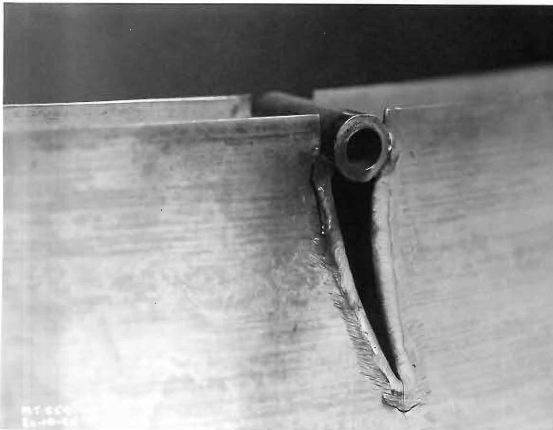
(b) CRACKS IN WELD ON OUTER WALL OF SNOUT
