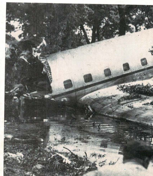
The crumpled fuselage of the Tudor rests in the partially drained pond providing a good illustration of the split in the forward fuselage. All photographs via Author
