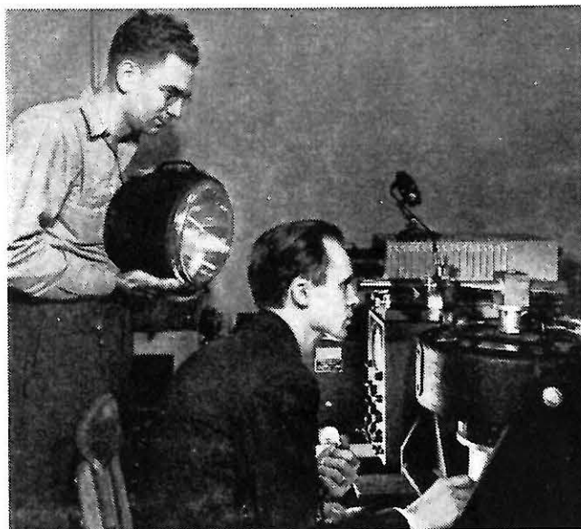
RIGHT: Vibration tests of turbine blades. Specialists are pictured using a high-frequency stroboscope lamp to observe a blade in motion on a powerful magnetic vibration.
