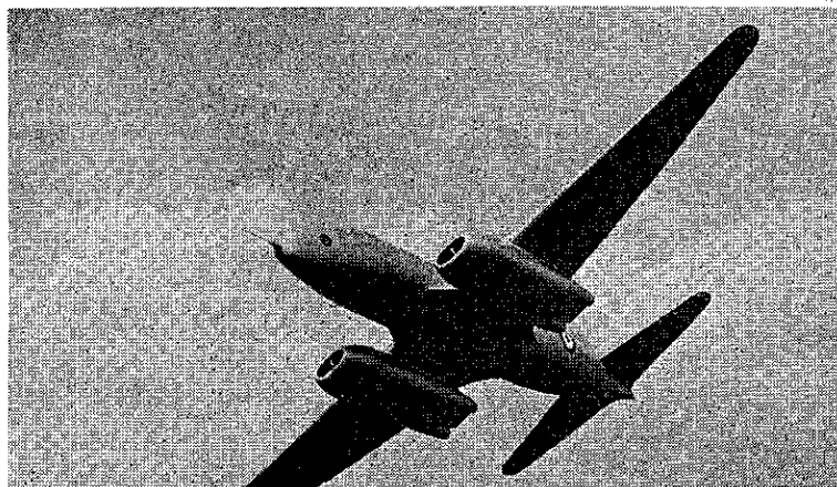
LOWER LEFT—One of the pioneers in British postwar flying research, the Armstrong Whitworth AW 52 "flying wing" has been investigating the problems of high speed flight with this type.
