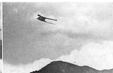
AS THE SEAT FLIES: Above, built for supersonic ejection, the new USAF "B" type seat is seen poised on its test launching platform on top of a supersonic rocket sled at Hurricane Mesa, Utah. Below left: seat is shown being rocketed forward and upward by its own integral rocket propulsion unit. At right, the seat is seen with the two telescoping booms which extend almost five feet out, provide more stability for the seat much as the stick on a sky-rocket.
