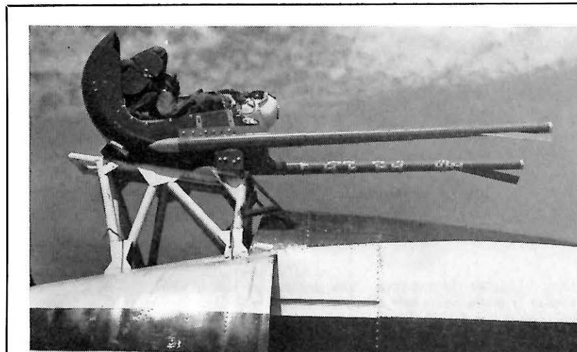
AS THE SEAT FLIES: Above, built for supersonic ejection, the new USAF "B" type seat is seen poised on its test launching platform on top of a supersonic rocket sled at Hurricane Mesa, Utah. Below left: seat is shown being rocketed forward and upward by its own integral rocket propulsion unit. At right, the seat is seen with the two telescoping booms which extend almost five feet out, provide more stability for the seat much as the stick on a sky-rocket.
