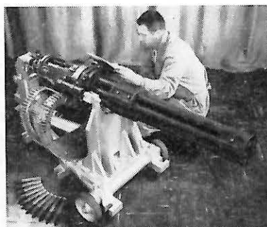
NEW VERSION OF VULCAN: The new 30 mm version of the Vulcan automatic cannon is shown above left alongside the earlier 20 mm version which is presently installed in the F-104A Starfighter. The new version, designated the T212, uses 50 percent larger shells and has three times the striking power of the 20 mm. Though it has shorter barrels, it weighs about the same.
