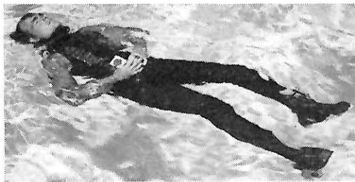
EXPERIMENTAL FLYING SUIT: New three-piece suit provides a number of advantages in supersonic era. It is waterproof, has a thermal liner for warmth, a ventilating suit for cooling, and is a partial pressure suit. It floats a pilot face-up, even when unconscious, with full gear and in cold water without undue exposure. It reduces by a third the time it now takes a pilot to don flying equipment, and decreases the bulk of equipment. Suit was designed by the Industry Crew Escapes Systems Committee for the USAF.
