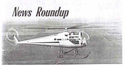
BRANTLY B-2 HELICOPTER is being distributed in Canada by Associated Equipment Co. FAF price for basic machine, Canadian duty and sales tax paid, is \$21,995. Powered by 180 hp Lycoming, the 1600 lb. B-2 carries two. cruises at 100 mph. Total operating cost is estimated at \$18.63 per hour.
