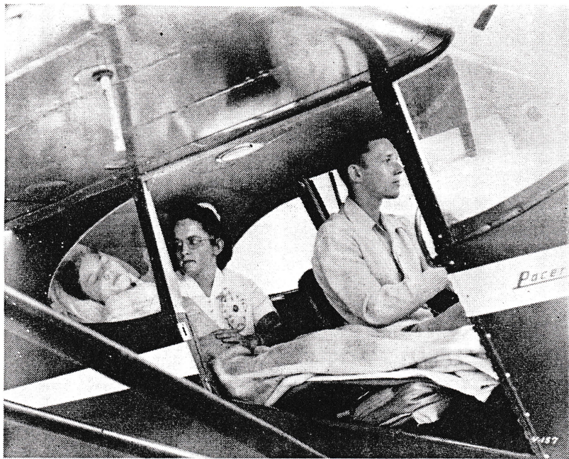
PACER AMBULANCE: The Piper Pacer may now be modified to carry out ambulance duties. By using a lightweight litter, the Pacer can carry a patient, a nurse, and the pilot. The litter is loaded through the left hand rear door with the foot placed on the right front seat after the back has been removed. The head of the litter rests on the back of the rear seat.
