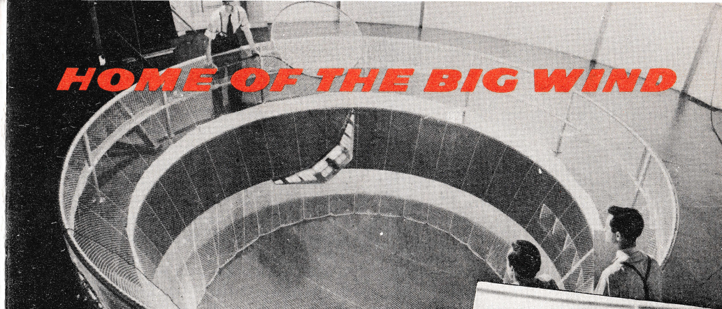
TESTING CANADA'S FLYING WING MODEL IN THE N.R.C.'S VERTICAL WIND TUNNEL NATIONAL FILM BOARD PHOTO
