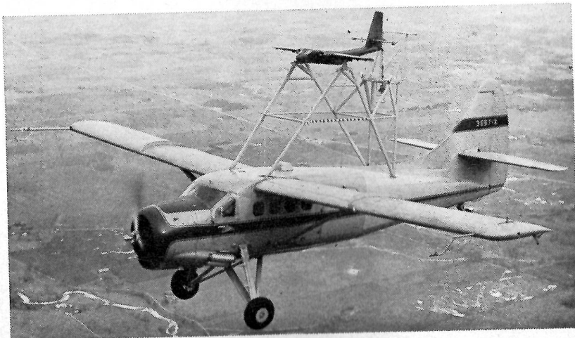
Above, the P & W R-2000 powerplant for the Caribou. Below, a Caribou scale model being tested under free flight conditions with the assistance of an Otter flying test bed. Technique is de Havilland developed.
