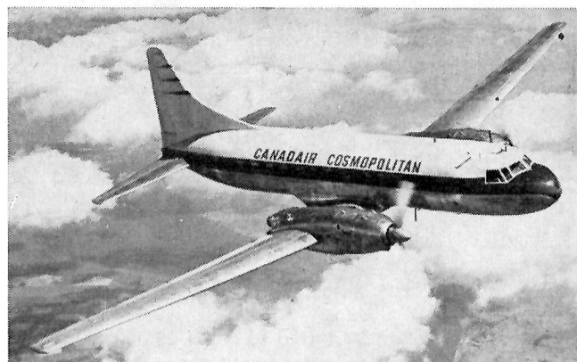
Photos show the original Convair 340 Liner which was converted to Eland turboprop power by Napier. Canadair CL-66 Cosmopolitan will be almost identical in appearance, but will be basically the later Convair 440 airframe.
