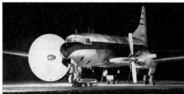
Photos show the original Convair 340 Liner which was converted to Eland turboprop power by Napier. Canadair CL-66 Cosmopolitan will be almost identical in appearance, but will be basically the later Convair 440 airframe.
