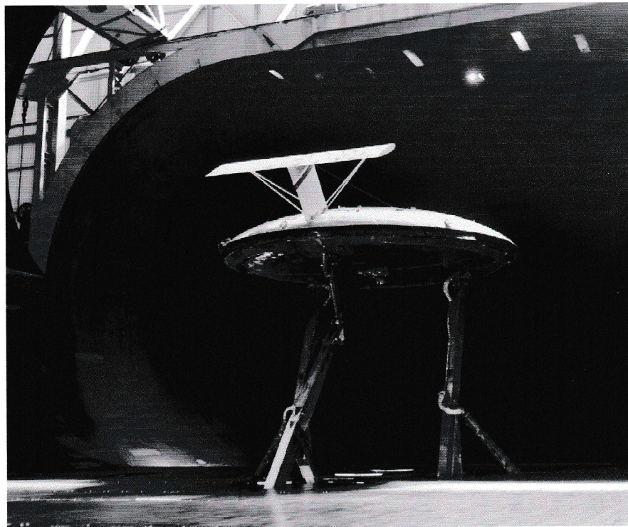
Figure 5. Avrocar (with tail) in NASA Ames Wind Tunnel
